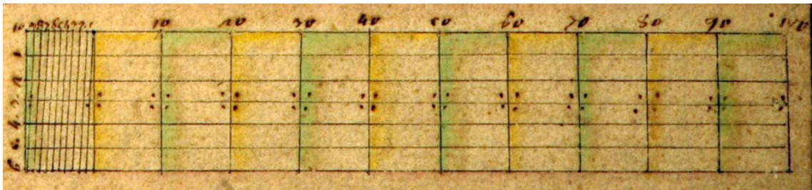
Figure 7 Tychonic scale of a Sabaudian cadastre, with the words "Scala di Trabucchi Centodieci". The scale has been build using the parameters b = 10 trabucchi, m = 6 and n = 10, so its accuracy is 1/6 trabucco or 1 Piedmontese feet, that is equal to 51.4403 cm. Note that the scale construction is inverted respect to the previous example
